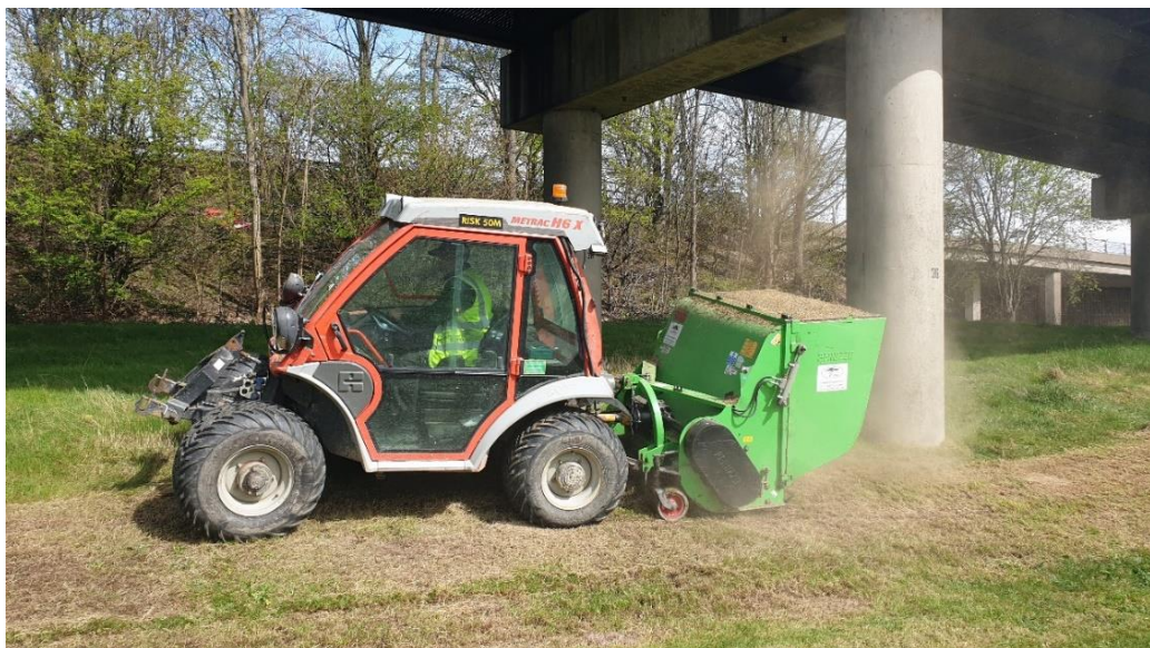
Reform bank tractor with mounted cutter and collection unit, March 2022 © Rachel Bicker
